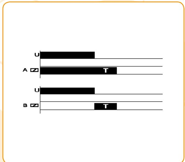
TRE 706 is a staircase switch. Time can be adjusted in the range from 0.5 to 10 minutes. It is edge triggered, which means that it is broken-switch proof. Enhanced version B has the possibility of multiplying ON time by factor 8. This fast-on function is activated by holding the switch for prolonged time (6- to 8 - second). This is very useful at cleaning, repairs etc.
