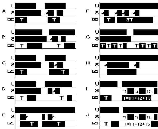
TRE 702 is a multifunction T1-T2 time relay with built-in microprocessor technology. It covers most of the user needs. The time relay comprehends simple and more sophisticated time functions with very wide time ranges. It can be delivered in many varieties according to operating voltages and the number of output contacts. It excels in the possibility of setting extremely asymmetrical T1-T2 time functions.
