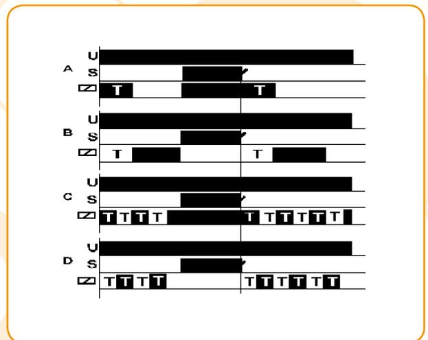
TRE 704 is a star-delta switch. Time T1 can be adjusted within the selected time range. It can be delivered in many varieties according to time range and operating voltage.
